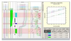
Production logging allows users to process and interpret spinner and fluid tools to identify volumes of fluid produced in their wells
