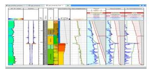
Pore pressure prediction outputs include results in pressure gradient and equivalent mud weight
