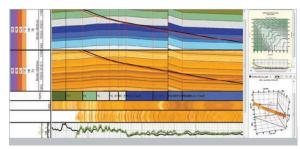
Geolog Geosteer allows an independent comparison of real-time log responses with a pre-drilling model, enabling monitoring of well progress and well plan modification if required.
