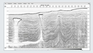
3D imaging of the SEG/EAGE salt model using Echos Reverse Time Migration
