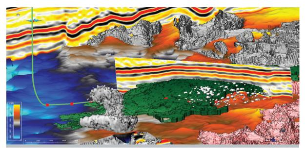
Integrated display of data in the Barnett shale (seismic, horizons, geobodies, karsts, wells and microseismic)
